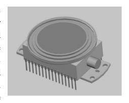
CCD 1024M has  $1024\times1024$  pixels (one pixel size is  $11\times11$  mm). CCD includes sections of accumulation and storage. The storage section has 1032 (V)×1048(H) elements format and independent of accumulation section control. The basic parameters are shown in Table 1.
